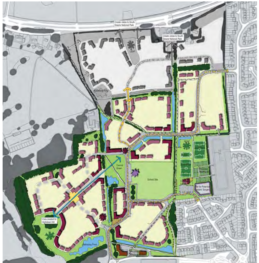
Figure 4.4: The Development Structure Concept Plan evolved the initial masterplanning proposals for the Application Site in more detail, highlighting key building frontages and a more considered network of principal roads.
