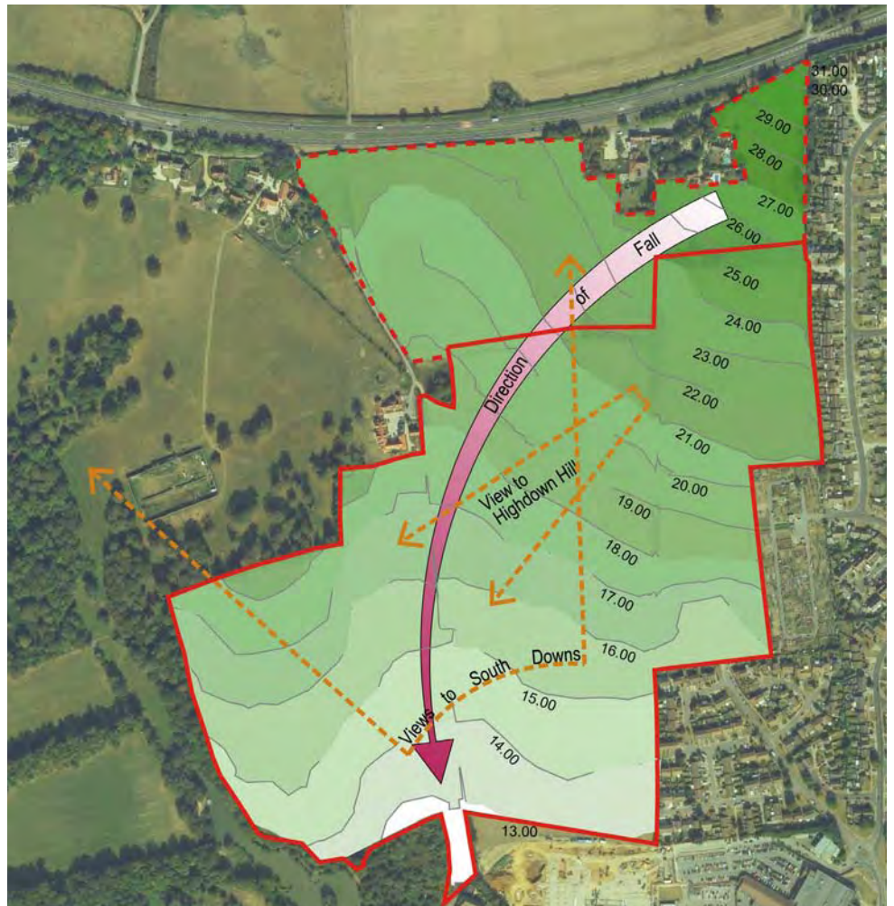
Figure 2.5: The Application Site slopes gently from the north east corner down to the southern boundary.
